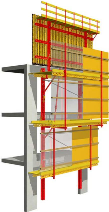
Figure 7: Climbing formwork with enclosed working platforms. (Graphic: PERI GmbH)
